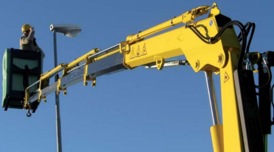
Thanks to the special "self-aligning" balancing system, the position of the basket is always horizontal without any intervention from the user.
