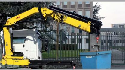
EES Extra Extension Speed SDS Smooth Descent System P-LCS Proportional Lift Control System LAS Liftrod Articulating System
