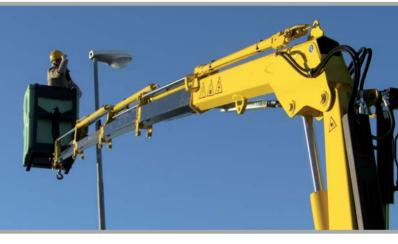
Thanks to the special "self-aligning" balancing system, the position of the basket is always horizontal without any intervention from the user.
