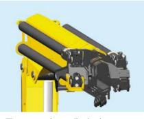
The extension cylinder layout has been designed to achieve compact boom and perfect alignment of the extensions.
