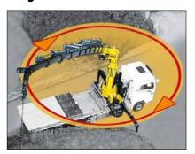
• Endless slewing allows the crane to be operated without restrictions. The complete access to the working area, eliminates the need to reposition the truck, optimizing precision, productivity and safety.
