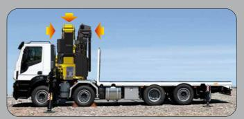
• Uniquely designed to reduce the space occupancy behind the cabin made for increasing payload and truck floor area.
