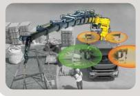
Detection and automatic activation of the operator's closest stabilizer. The Proximity Detection Module installed on each stabilizer allows to automatically activate the operator's closest stabilizer, avoiding potential human error.
