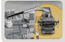
This system, a first on truck-mounted articulated cranes, optimises stabilization, makes crane operation safer and more efficient and allows the driver to verify in advance the crane lifting capacity based on truck stability.
