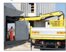
Negative angle between first/ second boom produces the most versatile crane structure available. The result is working flexibility - easier access to confined and low ceiling spaces.
