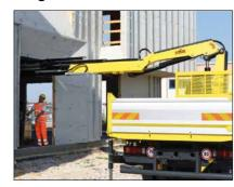
Negative angle between first/ second boom produces the most versatile crane structure available. The result is working flexibility - easier access to confined and low ceiling spaces.
