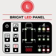
Available for the entire range till 28Tm. Highly user-friendly design, with buttons and LED lights. Dedicated led lights to identify the position of each stabilizer. New 3-digits display has been added to inform the operator about alarms and errors.
