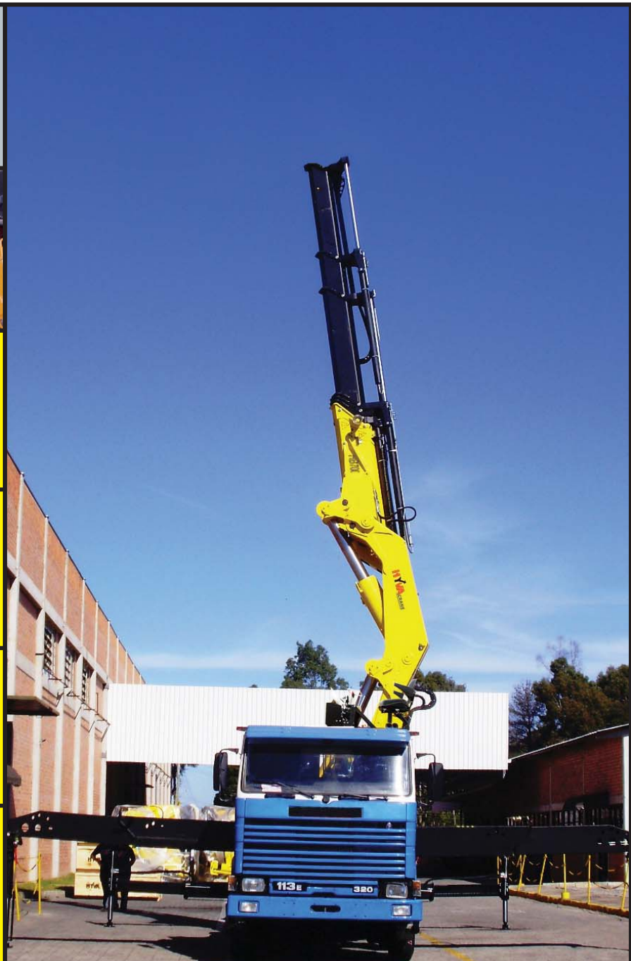
Second boom with negative angle in order to simplify operations in difficult access conditions
