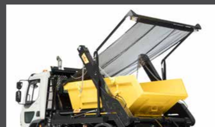
AUTO SHEETING SYSTEM
