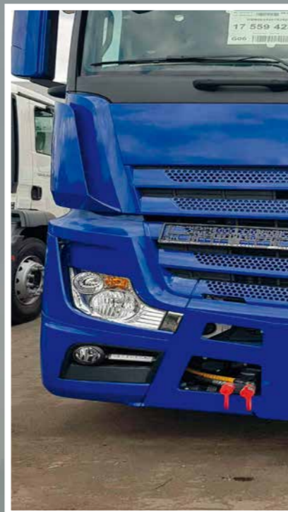
Quick release couplings in the front of the tractor
