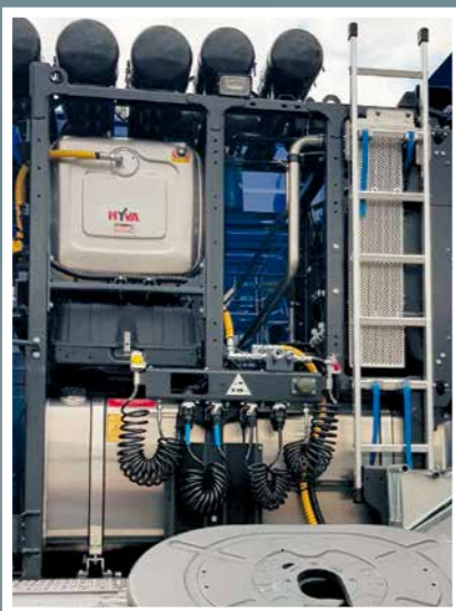
Oil tank behind cabin on 4 axle tractor unit
