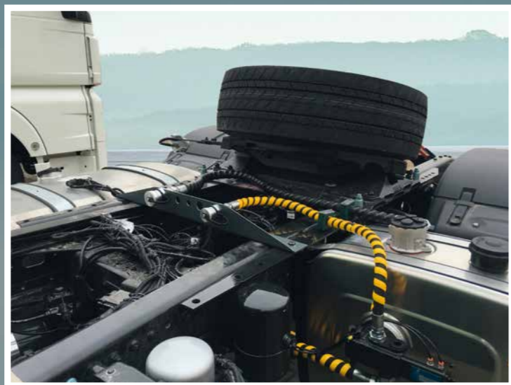
Mounting bracket for quick release couplings
