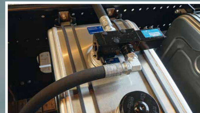
Tipping valve mounted on the return filter
