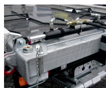
The balance of the lifting cross can be hydraulically adjusted.
