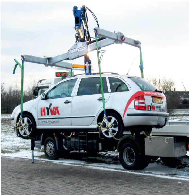
Adjustable wheel clamps with adjustable lifting ropes.
