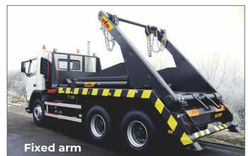
The steel platform is provided with two wearing strips in longitudinal direction. 6 adjustable container stops can be located through side steaks in the platform.
