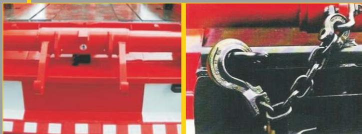
One tipping chain, length 650mm with open safety hook is mounted on the torsion tube. A second tipping chain or tipping hooks are available as an option.
