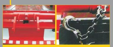
One tipping chain, length 650mm with open safety hook is mounted on the torsion tube. A second tipping chain or tipping hooks are available as an option.
