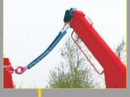
Walk on protection guards, for protection of the piston rod.
